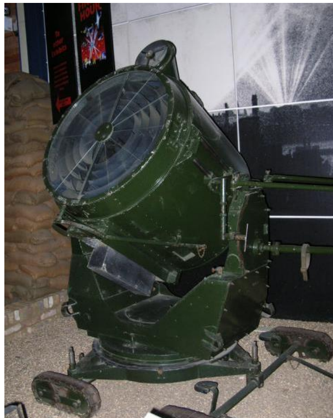
A WW2 searchlight in an RAF museum, showing the triangular base. The small tracked wheels were for moving it as in the photo above.
